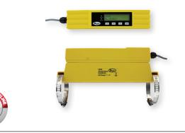
The **MODEL UFM** Compact Ultrasonic Flowmeters is an economical, clamp-on, ultrasonic flowmeter. The Model UFM implements the transit-time difference to measure flow rates in pipes and can measure velocity and flow in pipes with outside diameters ranging from 0.98 to 4.62" (24.89 to 117.35 mm). This model comes with a volume pulse and 4 to 20 mA flow rate output.
