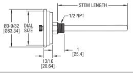
The SERIES BTM3 Bimetal Thermometer with Maximum/Minimum Temperature Pointer accurately measures the current temperature along with a maximum read or minimum read temperatures.
